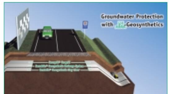
Considering various solutions, the regulators finally decided to install a GCL (geosynthetic clay liner) as sealing element. According to the calculations of the design office BBU in Braunschweig and the Bauberatung
