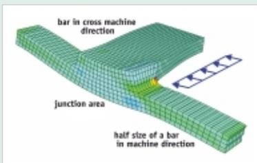
Junction deformation resulting from cross stress on the bar
