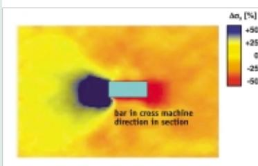
Pull-out test: Changes of horizontal tensions in a Secugrid® bar
